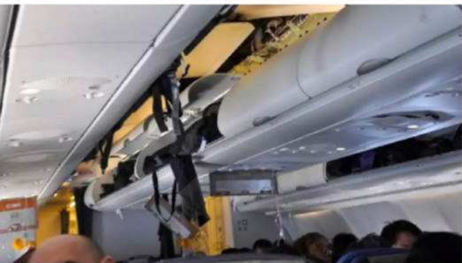
The force of the nosedives dislodged overhead compartment doors and ceiling panels.
